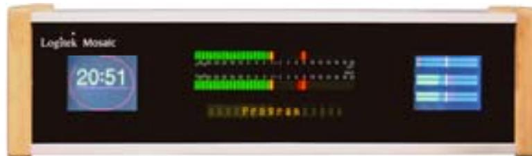
Figure 8 - Narrow Meter Bridge
